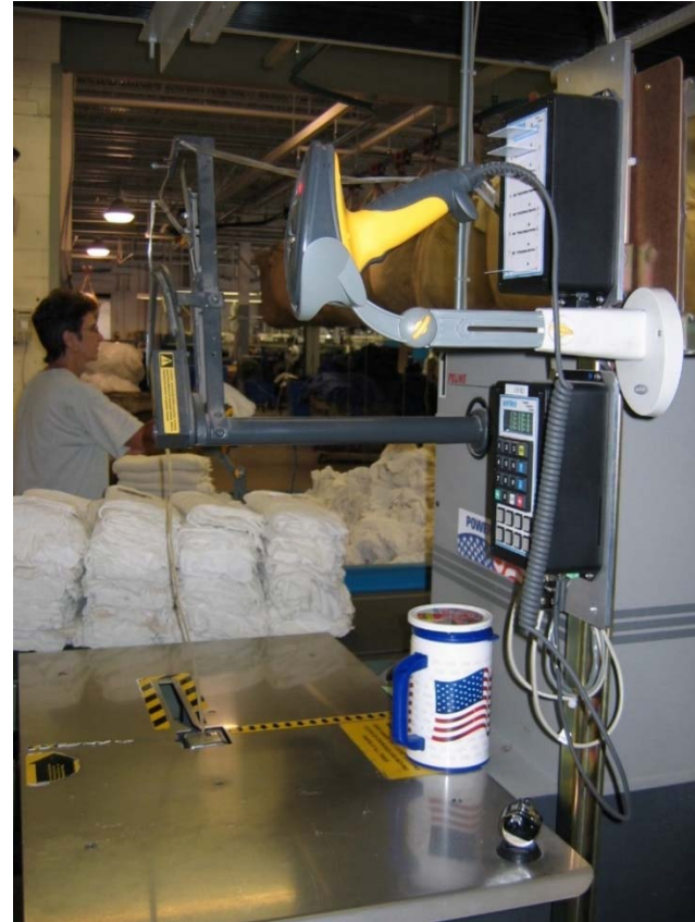
Classic PPS Box, 8 Card Reader Box, Audit Scanner & Tying Machine At End Of Belt
